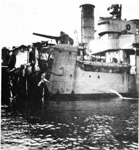
1 Another disaster: B.98 after striking a mine, October 1917. The sturdy construction of the B-Boats is proved beyond doubt 2 B.98 after mining, October 1917. She still manages to steam slowly ahead 3 Another view of B.98 after mining, October 1917 4 A bows-on view of B.98. A seaman can be seen standing amidships in the wreckage. (Bundesarchiv)
