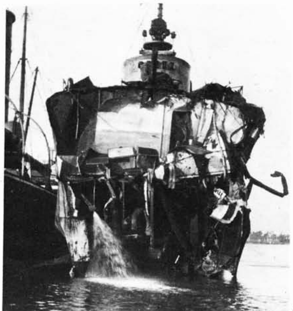
1 Another disaster: B.98 after striking a mine, October 1917. The sturdy construction of the B-Boats is proved beyond doubt 2 B.98 after mining, October 1917. She still manages to steam slowly ahead 3 Another view of B.98 after mining, October 1917 4 A bows-on view of B.98. A seaman can be seen standing amidships in the wreckage. (Bundesarchiv)
