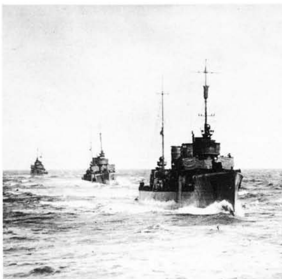
1 SMS Torpedo Boat B.110 in 1918 (Author's collection) 2 B-Boats in line ahead, 1918. The open bridges are protected by canvas dodgers. Note the propeller guard on the starboard quarter (Author's collection) 3 B.110 leads the line (Courtesy Serge Pillar)
